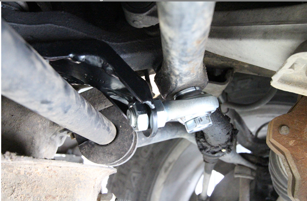
Figure 3: Idler arm bracket installed
