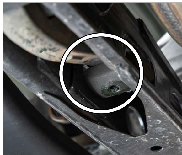
Figure 1: Measure and Remove Torsion Bar Adjuster Screw
