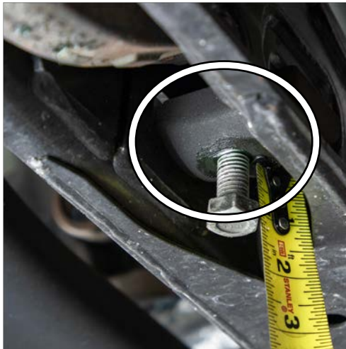
Figure 1: Measure and Remove Torsion Bar Adjuster Screw
