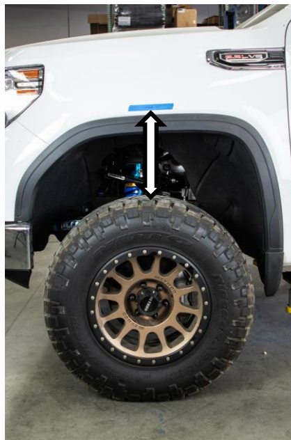
Figure 6: Measuring and Setting Ride Height
