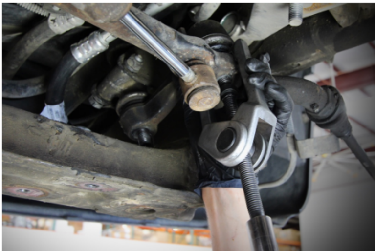
Figure 2. Remove center link with puller.
