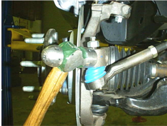
Figure 1. Remove tie rods from spindles.
