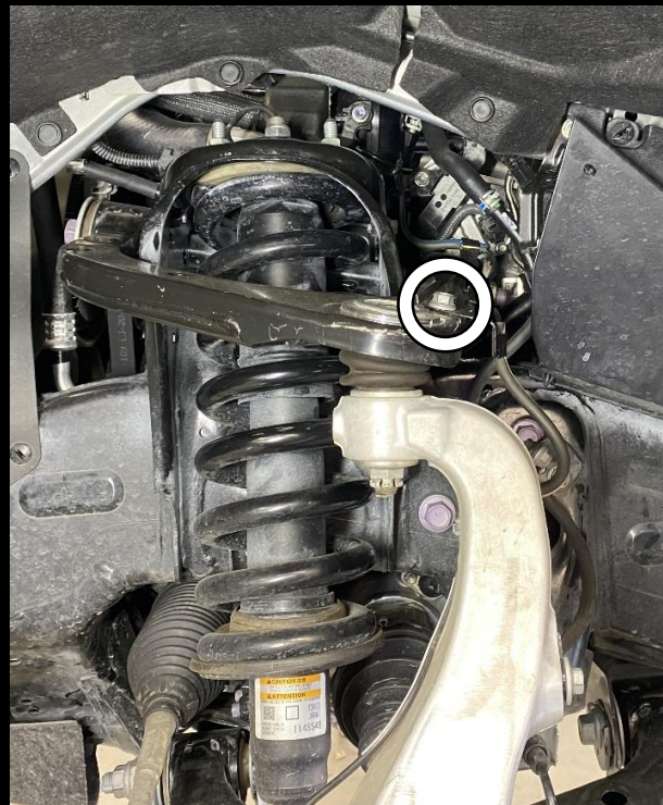
Figure 6: Remove ABS bracket from upper control arm.
