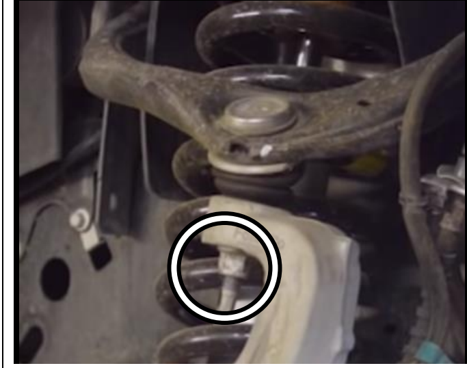
Figure 2: Upper Ball Joint Pin and Spindle Removal
