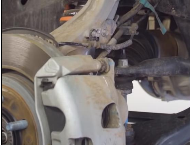
Figure 1: Sway Bar End Link Removal
